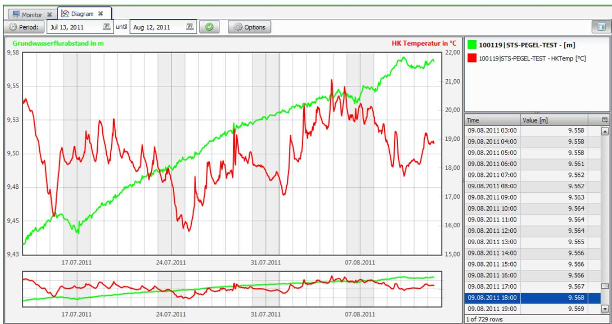
The diagram shows in a dynamic scaling the values of the defined period of time and the chosen sensor channel of the device list. The lower diagram is used as an overview window, while you can zoom in the upper diagram. To zoom-in into the diagram please left-click and hold the mouse button to draw a rectangle. You can draw one in the upper and lower overview.
