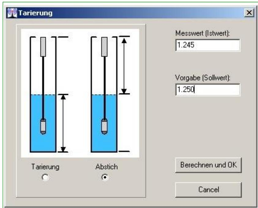
In both cases you need to have the Values to be measured (Set-Point). The value actually measured by the Device is known, too. If you executed a measure, the Just-Value is put into Field Just-Value by the Shell-Software; for Example 1.245 Meters.
