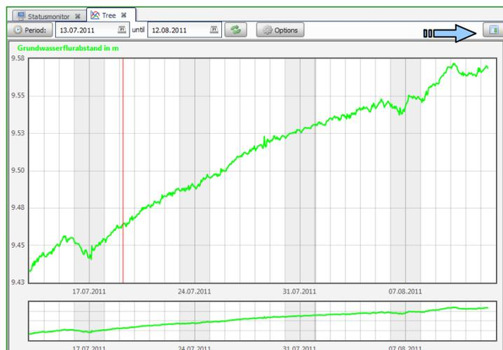
The online portal offers you the possibility to display two measuring values in one diagram. To do that please choose two values within a device of your sensor network. To switch between the measuring values click on one device entry in the upper right window.
